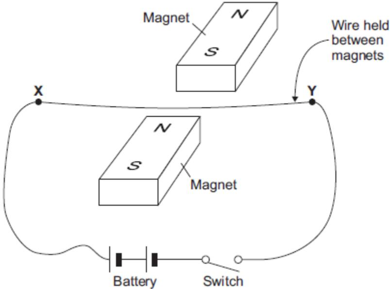
Closing the switch creates a force that acts on the wire **XY**.
