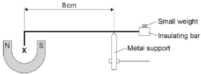
The wire **X** is 5 cm long and carries a current of 1.5 A.
