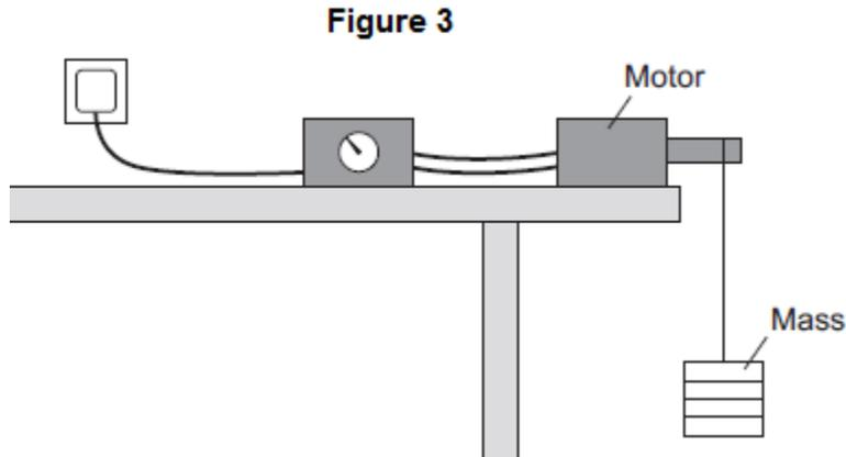
The student varied the electrical input power to the motor. For each different electrical input power, he recorded the time taken to lift the mass and calculated the output power of the motor.
