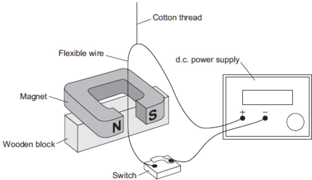
When the switch is closed, there is a current of 2 A through the wire. The wire experiences a force and moves.
