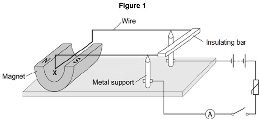
When the switch is closed, the part of the wire labelled **X** experiences a force and moves downwards.
